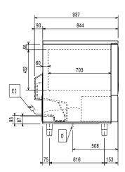
Drain Electrical inlet (power) ΕI Refrigerant Outlet
